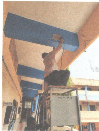
Fig. 3. Ultrasonic Pulse Velocity Test on beam
